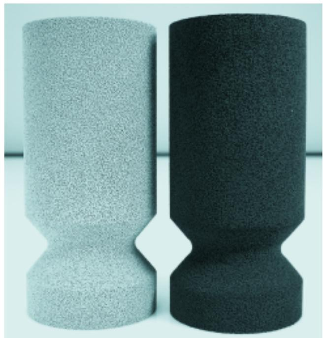
**Figure 7. Silicon Carbide Foam Thrust Chamber Core Shown on Right; A Molybdenum Foam Core is Shown on Left.**
