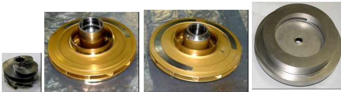
Figure 8. Hydrogen pump parts of powder alloy (inducer, first and second stage impellers, distributor blank)
