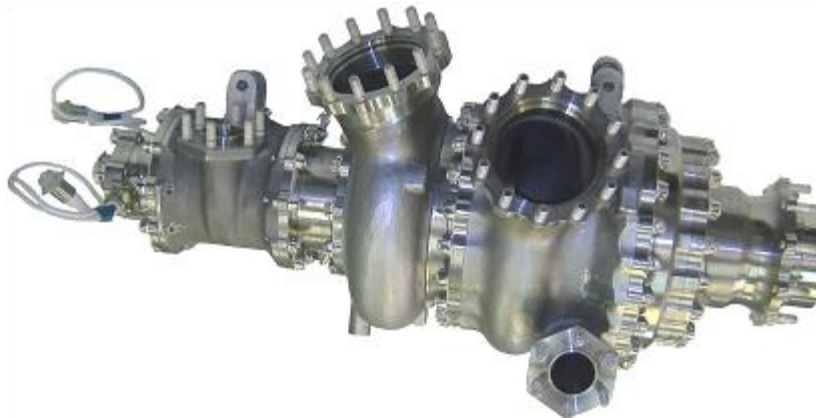
Figure 5. Single shaft TPA of RL10 engine
