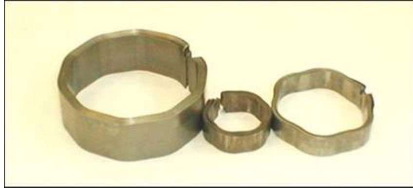
Figure 7. Plate-type corrugated elastic elements
