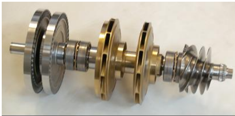
Figure 6. Rotor of single shaft turbopump hydrogen pump
