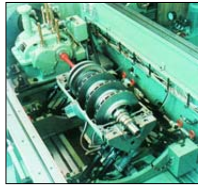
Figure 5. RD-0120 Engine Rotor on Spin Balance Test Stand.
