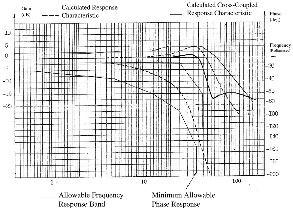
**Figure 8. Simplified Closed-Loop Frequency Response Including Additional Feedback Control (Velocity, Differential Pressure, etc)**
