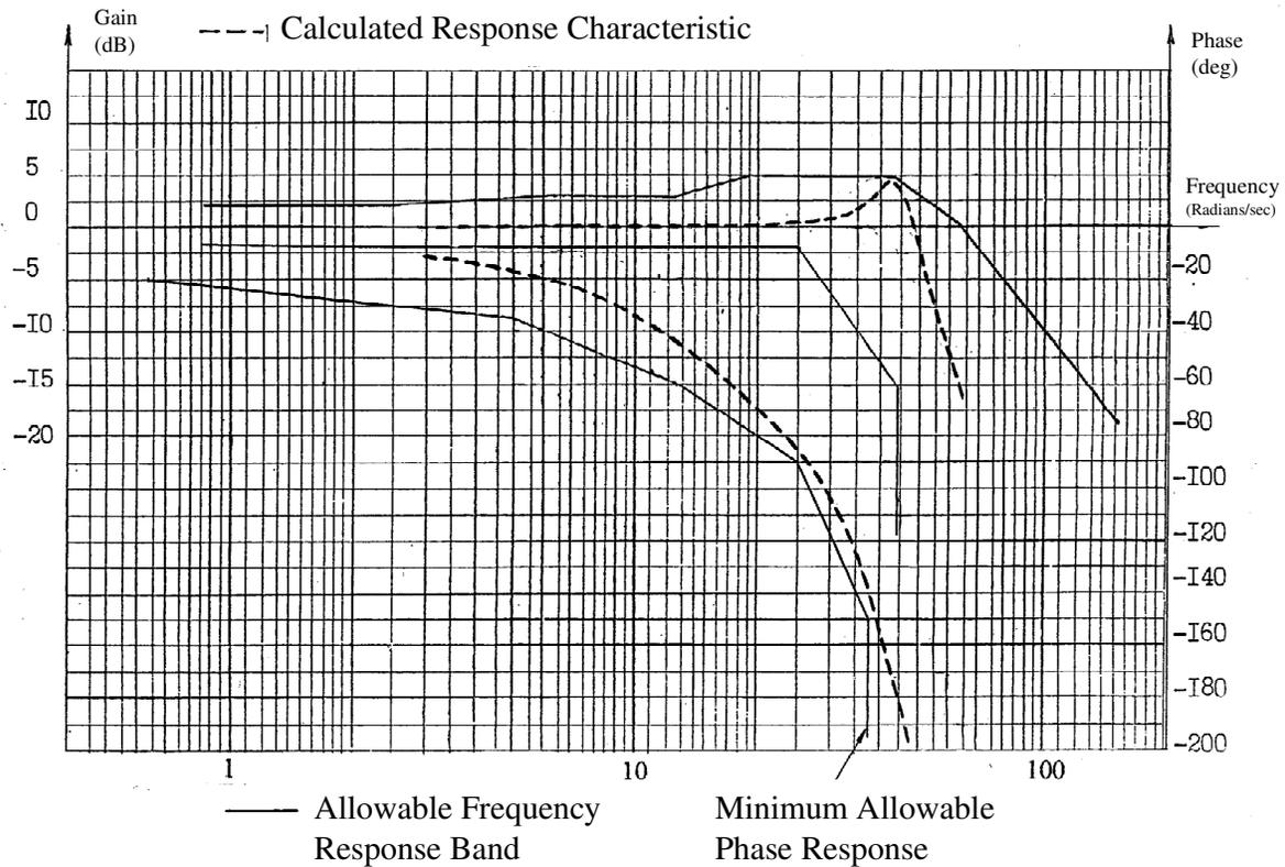
**Figure 7. Closed-Loop Frequency Response without Additional Feedback Control (Position Feedback Only)**
