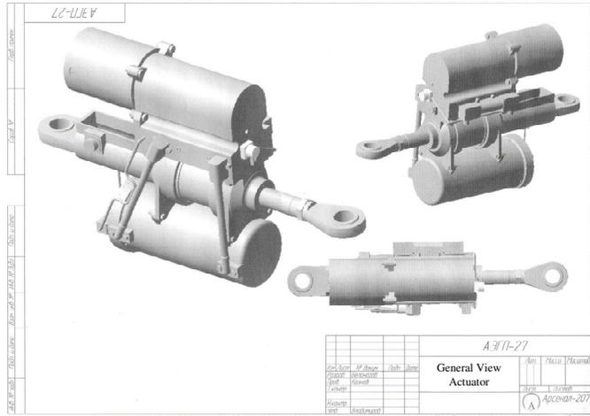
**Figure 6. General View of EHS with an Output Power of 225 kN**
