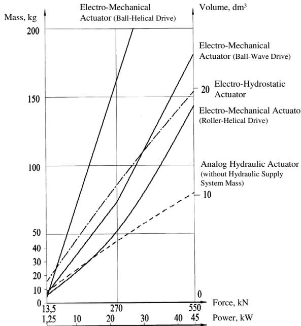
**Figure 2. Actuator Volume and Weight vs. Actuator Force for Three Actuator Types (Actuator Velocity of 300 mm/sec)**
