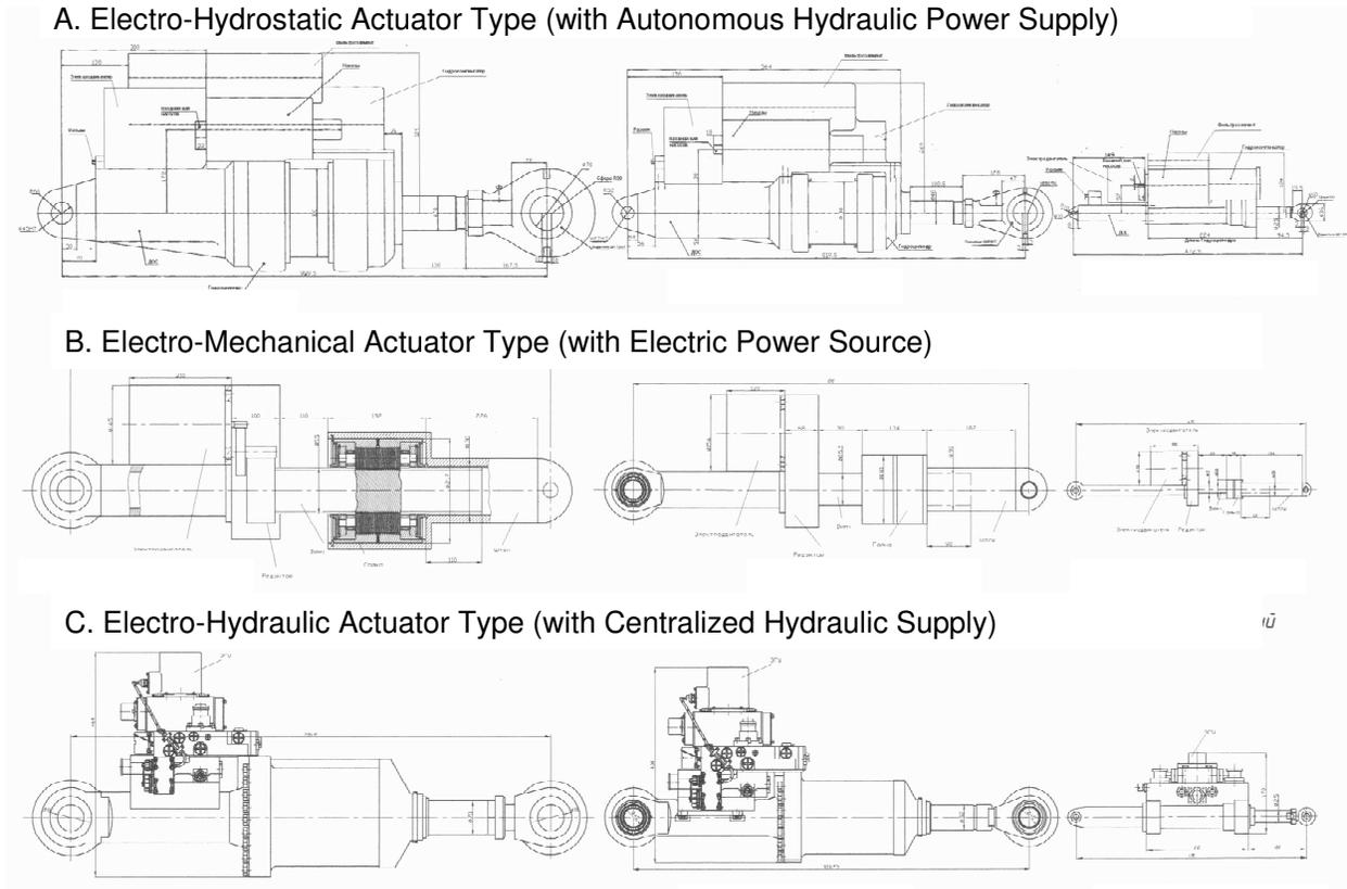
**Figure 1. Comparison of Different Linear Actuator Types for Three Different Actuator Power Outputs – A. Electro-Hydrostatic, B. Electro-Mechanical, C. Electro-Hydraulic**
