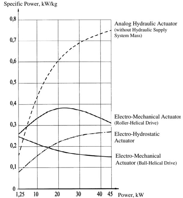
**Figure 3. Comparison of Specific Power vs. Power Output of Various Actuator Types**
