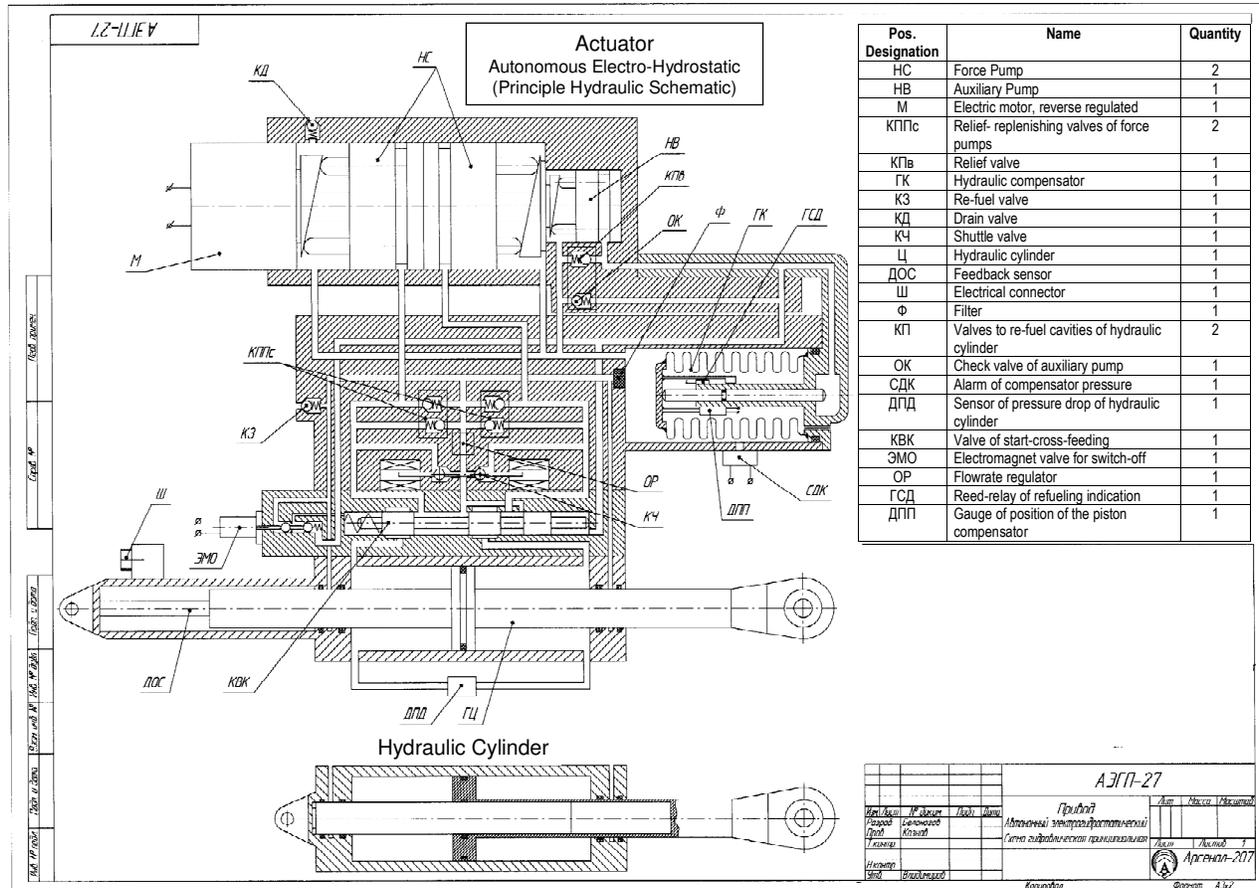
Figure 4. Simplified Schematic of Electro-Hydrostatic (EHS) with Self-Contained Auxiliary Pump
