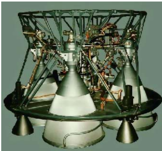
Figure 2. External view of the RD-0110 engine.
