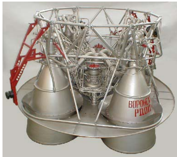
Figure 3. External view of the RD-0124 engine.
