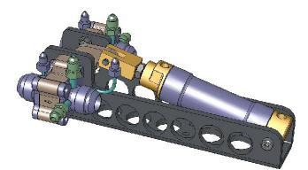
Figure 4. Ganged-actuator LOX-fuel valves with purge and igniter tapoff ports, using COTS cryo-rated valve components.
