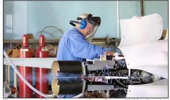
Figure 11. Mechanic wearing face shield, hearing protection and gloves loads liquid oxygen into EZ-Rocket.
