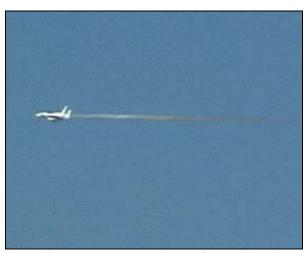
Figure 2. EZ-Rocket dumping LOX during intact abort, Flight 11. (Image from video capture.)
