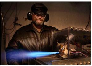
Figure 3. Oxygen-kerosene igniter during statistical testing (note shock diamonds in plume).
