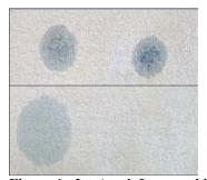
Figure 6. Jet-A, left, vs high grade kerosene on right. High grade kerosene evaporates completely in 10-20 minutes.
