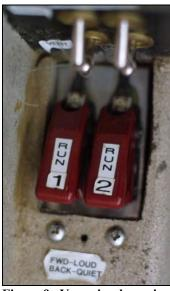
Figure 9. Very simple engine control interface for pilot.
